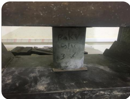
Fig.5: Specimen under compressive strength test
