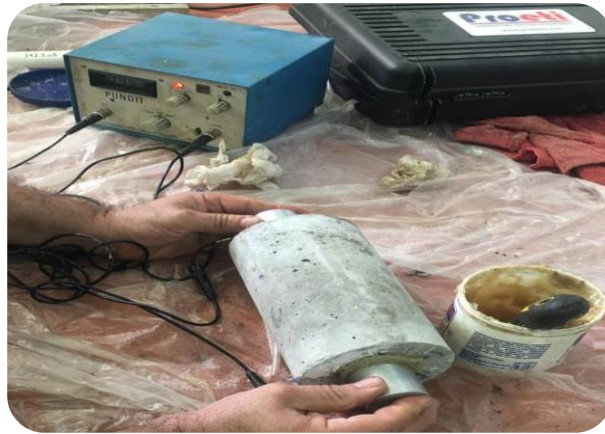
Fig.7: Pulse velocity of the concrete specimens.
