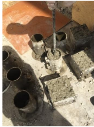
Fig.3: Compacting using a tamping rod.
