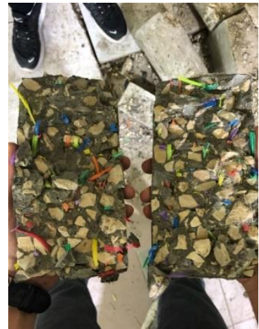
Fig.12: Fiber distribution after testing for PS-0.5 sample
